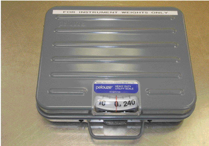
Photo2: Scale used to weigh instrument sets.
